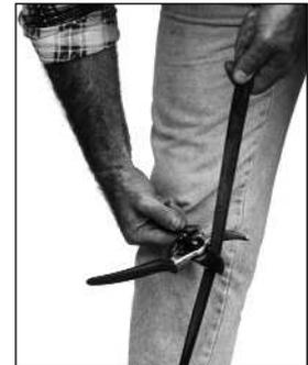
*Step 4.* A fine burr will develop on the edge of the flat side of the blade. When it does, stop sharpening. Remove the burr by using the stone in light, slow careful circles. About 5-6 circles should be sufficient. Make sure you do this with the blade at a shallow angle of about 5 degrees. Alternatively, use a narrow leather strop (an old belt) to remove the burr.
