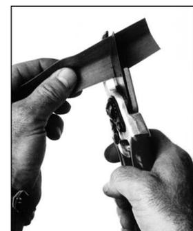
*Step 4.* Oil and assemble all the parts. Adjust the tension on the pivot screw so that the blade and the anvil slide past each other with no gaps and without jamming. You can easily hear the blade and anvil slide past each other *without* putting them anywhere near your ear. (Don't become a Van Gogh!)
