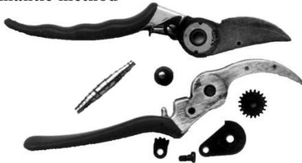
*Step 1.* Remove the spring and pivot screw. Clean all parts before you sharpen the blade.
