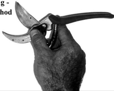
*Step 1.* Open the secateurs wide. Grip the secateurs in your right hand (or left hand if using left-handed secateurs). Rest your thumb on the pivot screw. Use your index finger and palm to prop open the handles. Use your 2 middle fingers to hold the secateurs firm.
