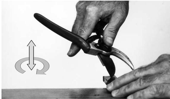
*Step 3.* Hold the stone firmly. Rotate the secateurs clockwise (or anti-clockwise) lifting your elbow to sharpen the tip of the blade and lowering again to sharpen near the pivot. This action sharpens the whole blade evenly without creating any flat spots. A smooth even action is important. Be careful when near the pivot not to damage the anvil.
